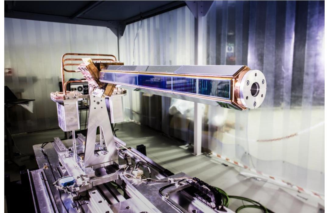
Si-array consists of DSSD's for detecting protons
