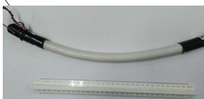
SPND detector with mineral cable INTC-I-247 Acknowledgement: S.Fiore EP-UNT
