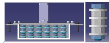
Replace 2 samples holders by with square boxes (allow different samples shapes) Acknowledgement : C.Mucher, L.Buonocore and M.Macha SY-STI
