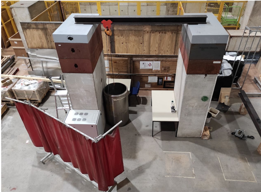
Figure 3. Left and middle: the dewar with inner dimensions 70 cm diameter and 120 cm height. Right: 3D model of the entire dewar setup
