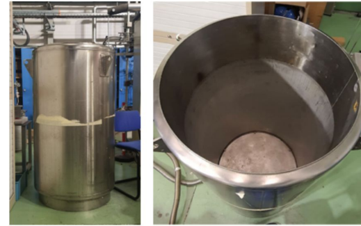
Figure 3. Left and middle: the dewar with inner dimensions 70 cm diameter and 120 cm height. Right: 3D model of the entire dewar setup
