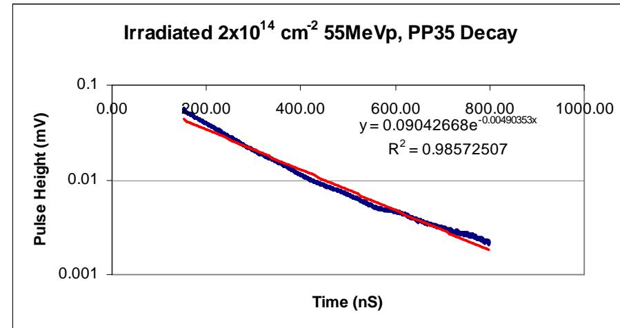
Time Const= $R * (C + C_{3d}) = 177 \text{ nS}$ ,  $C_{3D} = 91.6 \text{ fF}$
