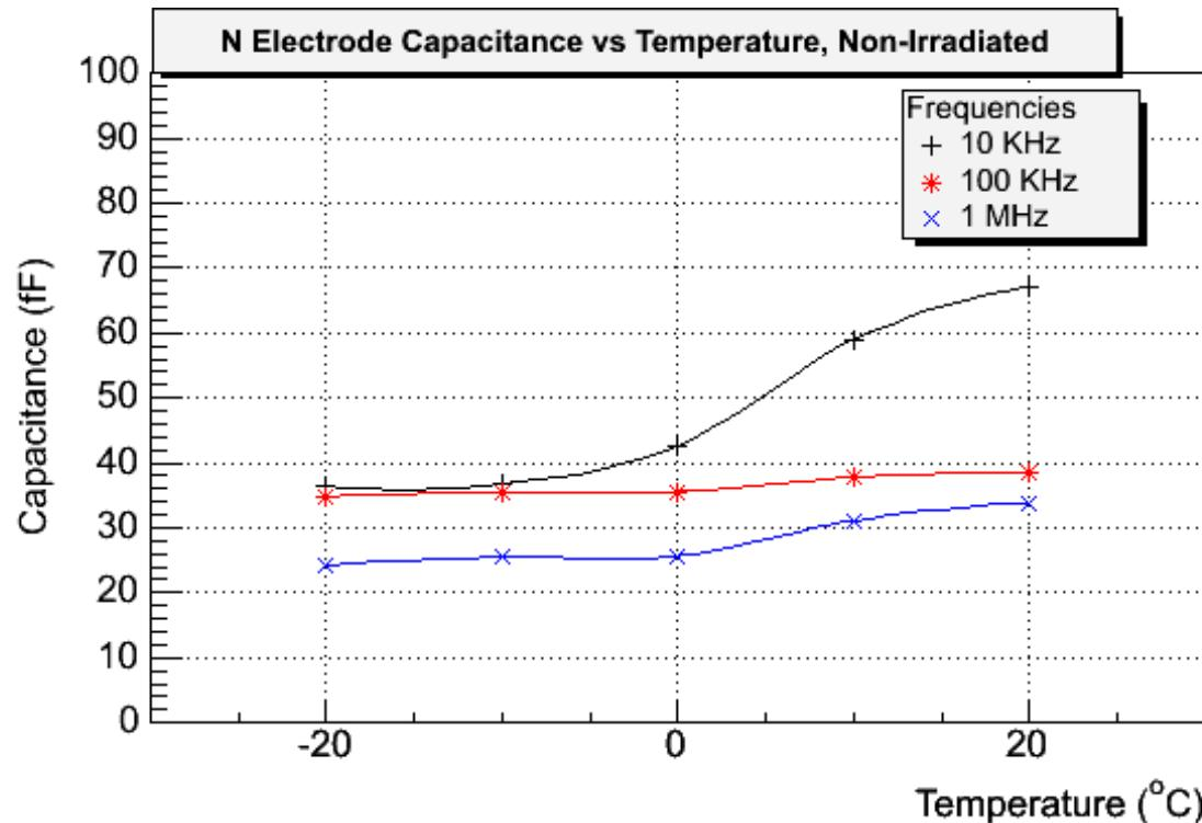
**Result: electrode capacitance decreases with lower temperature, and reaches a minimum value at ~ -10°C.**
