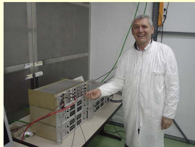
Picture 9: Dr. Sandor Czellar beside four high voltage power supplies and a trigger box he has developed and manufactured for the Finnish Cosmic Rack. Similar PVs and Trigger Systems are used in CMS Tracker module testing centers.
