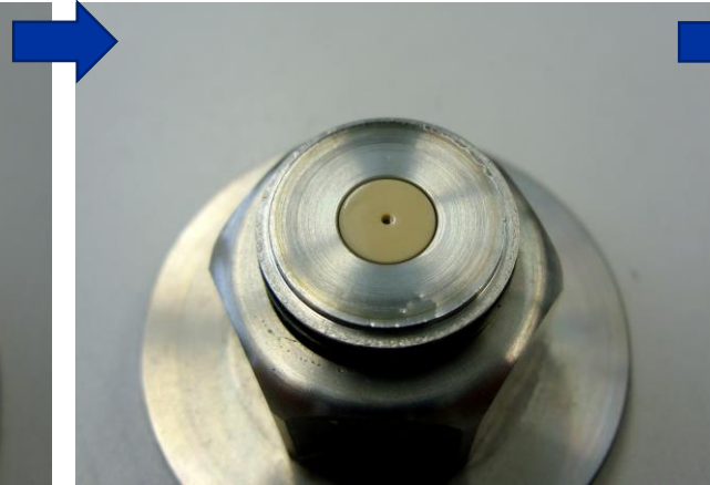
Membrane removed Discoloration of sintered ceramic
