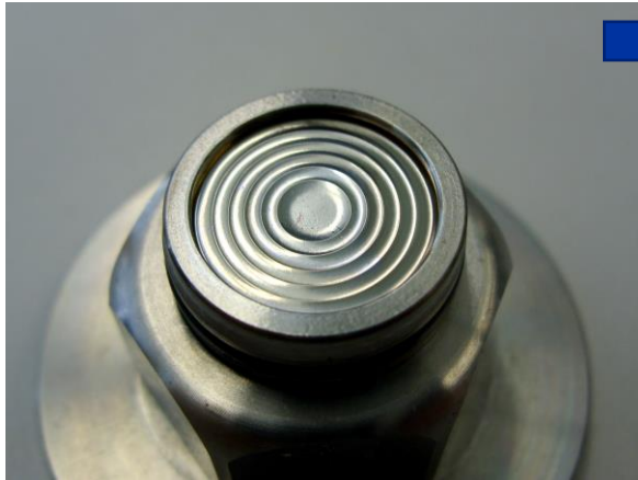
Stainless steel membrane in normal condition
