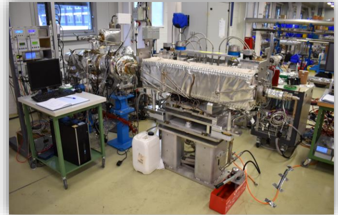
Vacuum acceptance test of spare TCTPV in bldg.867
