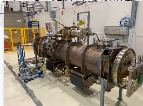
Acceptance test of the MKI cool in Bldg. 867
