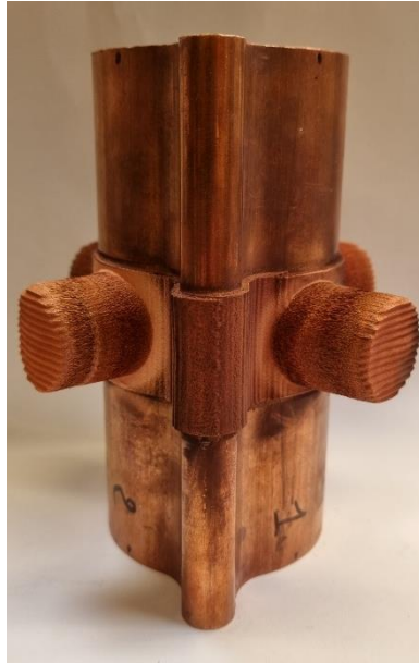
Chamber prototype with x4 bosses for direct BPM buttons machining and SMA rings
