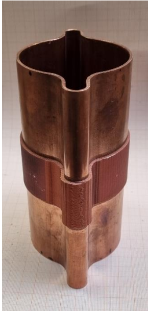
Chamber: 2mm layer sprayed all around
