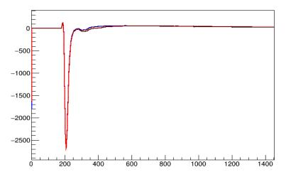
Average gamma-flash response of an empty cell for the two different gases used (Ar: $CF_4$  with 2% (blue line) and without (red line) iso $C_4H_{10}$ )
