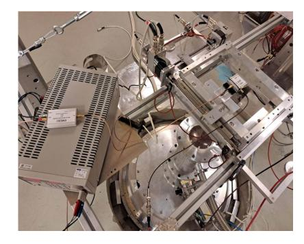
In the EAR-2 tests last November, two DC amplifiers were tried Micro (10mV/µA) and Nano (10mV/nA) to cover a large range of neutron energies. Nano amplifier is much slower than Micro
