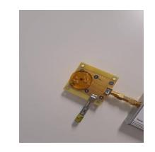
The diamond detectors (4 mm x 4 mm x 50 µm) have been developed and produced by CIVIDEC Instrumentation. R&D for the electronics of diamond active detector to measure the neutron fluence at the n\_TOF NEAR station.
