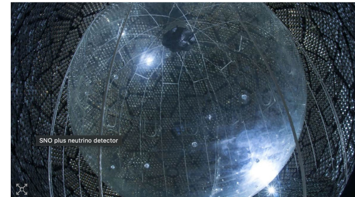
Reactor reactions: the SNO+ detector has seen antineutrinos from distant reactors when it was filled with pure water. (Courtesy: SNO+)
