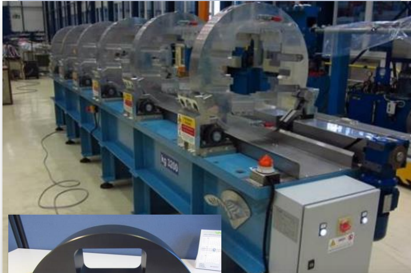
Rotating Table for SC magnets assembly
