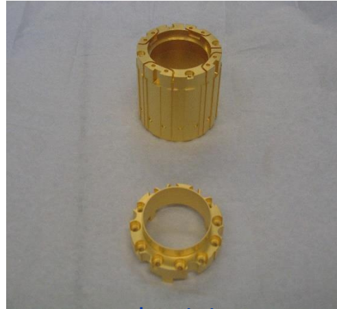
Magnets aluminium parts + gold coating
