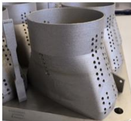
As-built surface Surface brute de fabrication
