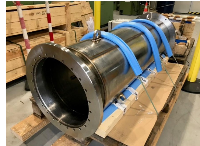
Cryocooler Test Chamber
