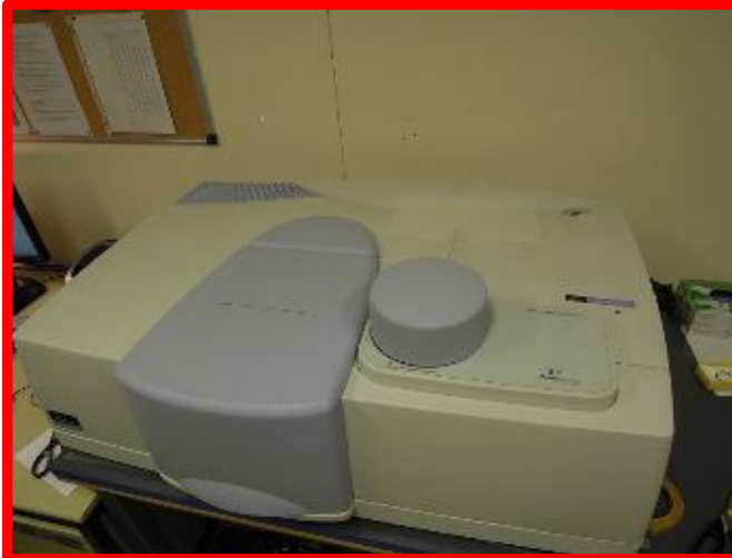
Perkin Elmer spectrometer for spectral/diffuse reflection and transmission (200-900nm)
