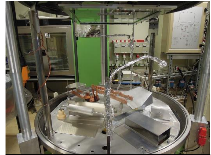
AR quartz window for LHCb RICH1
