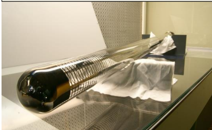
Titanium (conductive) spirals on CLOUD UV sabre
