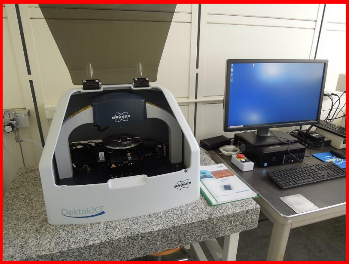
BRUKER Profile-meter DEKTAK for measurement in nm scale
