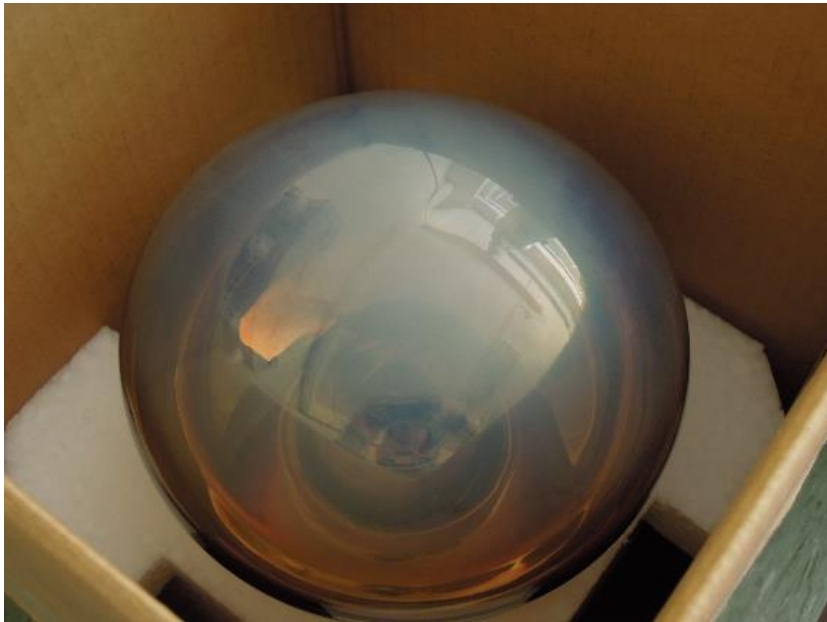
PM wavelength shifter coating (TPB)
