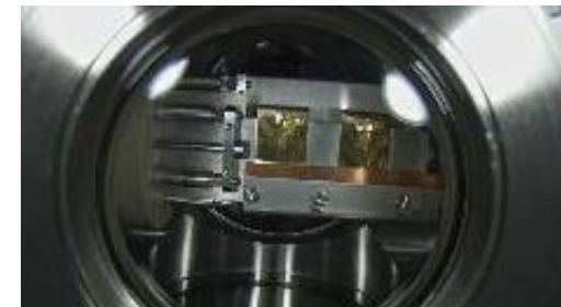
Zinc layer on gold plates for MEDICIS (Medical Isotopes Collection ISOLDE)
