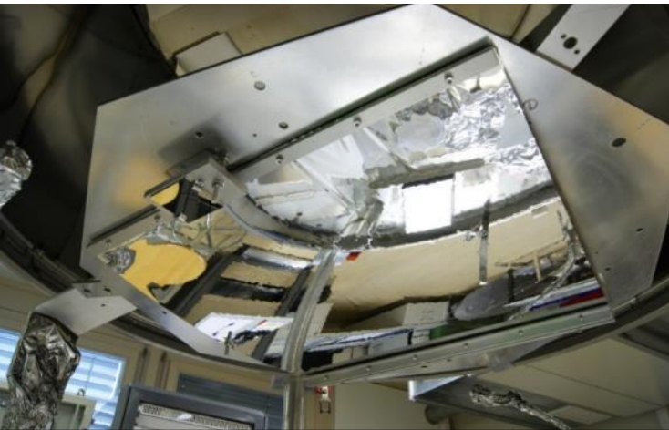
Mylar foil coating for NA62 RICH optical feed trough
