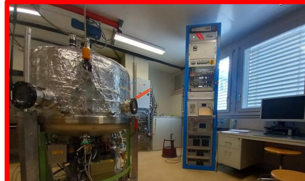
Upgrade big production coater (1m diameter)
