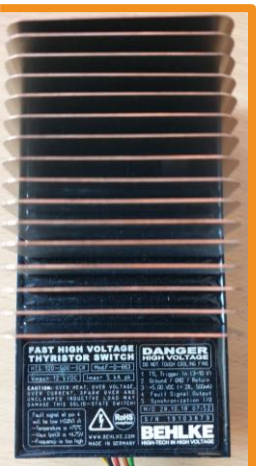
HTS 120-500-SCR old switch with integrated trigger module
