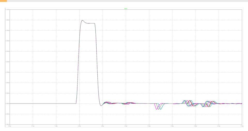
Simplified LTSpice simulation for storage cable lengths of 195 m, 200 m and 205 m with transmission lines: 65 m, 67 m, 70 m, 74 m, 76 m
