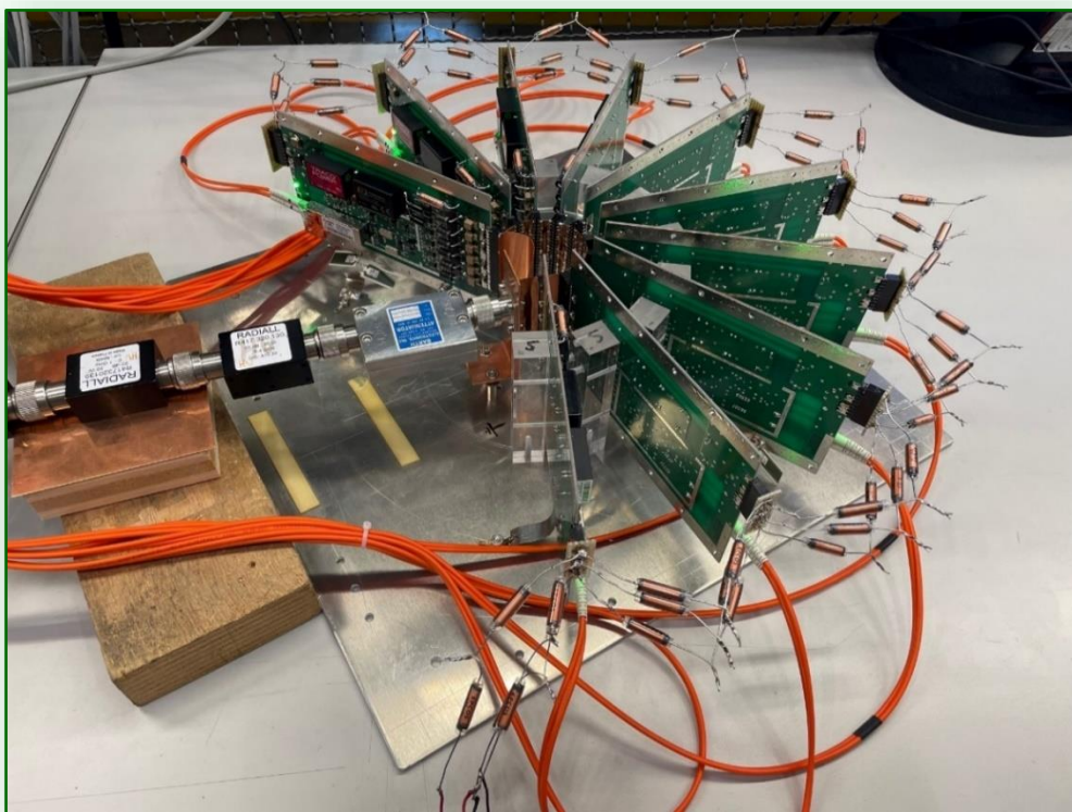
10 stage GaN FET based pulse generator
