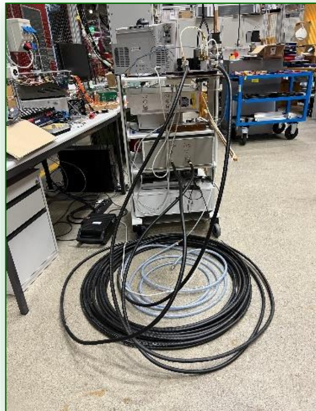
Measurement setup with 20 m cables - for pulse generator protection
