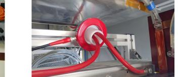
Measurements in laboratory environment to validate the scope signals of pulse current and ground fault current.
