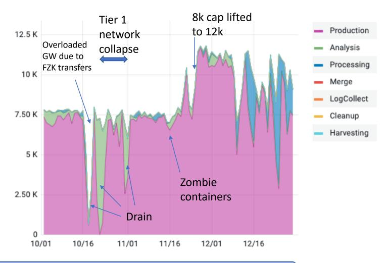
A few periods of production job drain in second half of October due to failing webdav tests (T1 legacy network collapse etc.)
