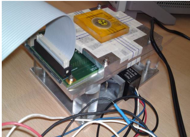
Figure 6 : A sr-90 source aligned above the silicon detector with an aligned Scintillator trigger below.
