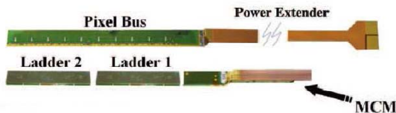
Figure 1 : Sketch of the half-stave assembly: the two ladders (5 readout chips each) and the MCM.
