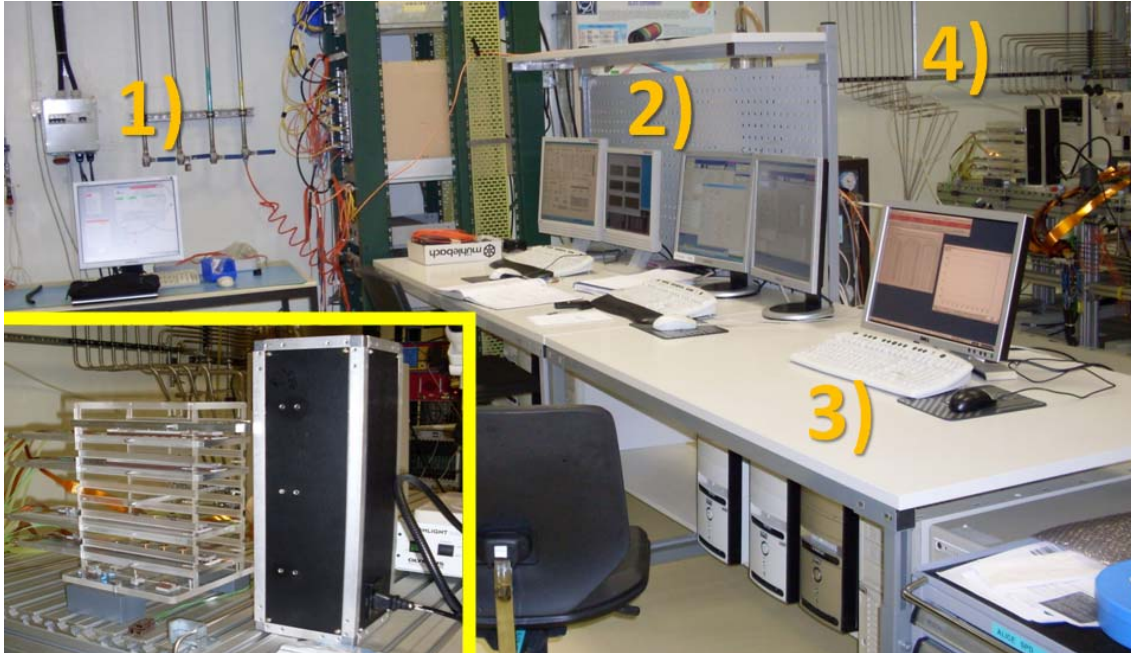
Figure 5 : A schematic view of the apparatus. 1) DAQ station, 2) DCS station, 3) Online monitoring station and 4) Planes containing the ALICE pixel detector half-staves. The bottom left picture shows a detail of the 4 planes with the 4 half-staves and the cooling (black box).
