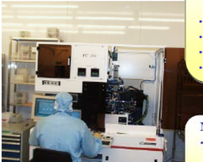
Suss MicroTec FC150 Flip Chip Bonder with both Universal and Solder Reflow Bonding Arms.
