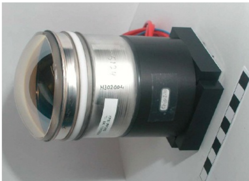
8192-channel pixel chip 8× OR → 1024 pixels (500 × 500 μm square)
