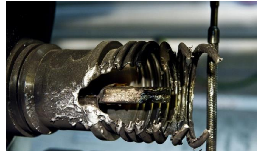
Joint failure damaged 50 magnet
