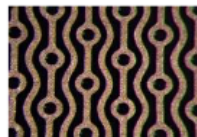
Figure 2. A single-phase TPC with a L-MHSP (or L-COBRA, shown) coated underneath with CsI. Ionization electrons and UV-induced photoelectrons from CsI are collected into the L-MHSP holes, and drift towards the anode strips. VUV photons emitted by EL + small avalanche near the strips, are detected by the top photo-sensors. Another fraction of S1 photons are detected by bottom photo-sensors.
