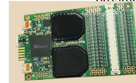
example discrete electronics pre-amp-shaper-pulser-trigger
