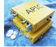
example discrete electronics pre-amp-shaper-pulser-trigger
