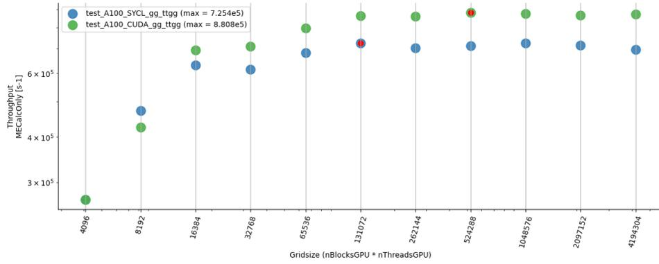
SYCL vs CUDA throughput for gg\_ttggg on Nvidia A100
