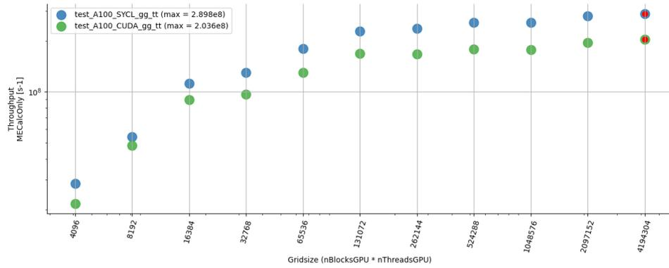
SYCL vs CUDA throughput for gg\_ttg on Nvidia A100
