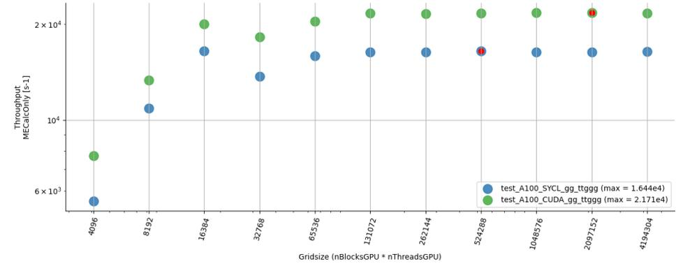
SYCL vs CUDA throughput for gg\_tt on Nvidia A100
