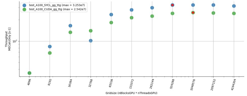
SYCL vs CUDA throughput for ee\_mumu on Nvidia A100
