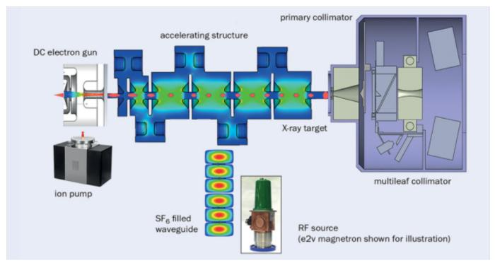
**Linac essentials** A standard medical linac comprises an electron gun, an accelerating structure, a target and a collimator. Also needed are an RF source to power the linac, a waveguide to transport the power between the linac and the RF source, and a vacuum pump to keep everything under vacuum. Credit: D Angal-Kalinin/G Burt/M Dosanjh
