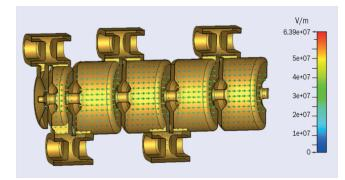
**Strong coupling** The ITAR linac cavity geometry showing the electric field contour map, with the short first and second cells, and strong coupling to the first
