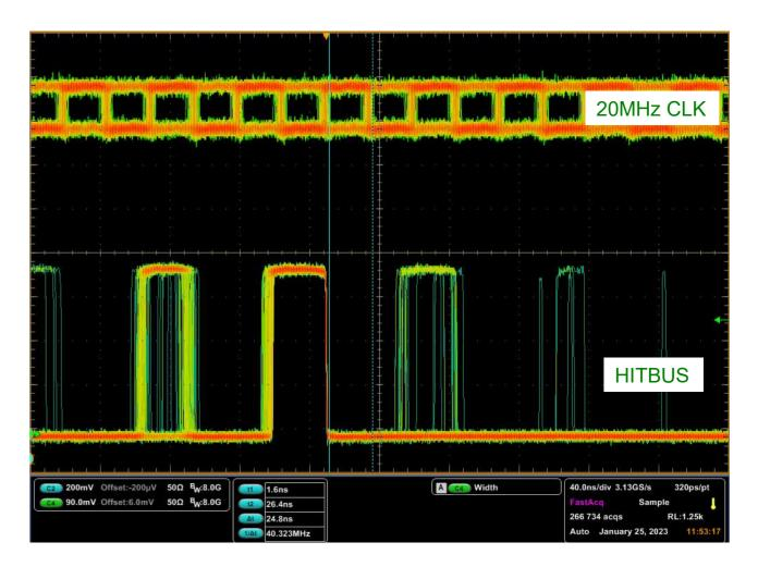
Signal on SFOUT only when COMP detects signal (TH low)
