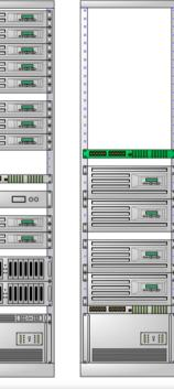
CPU: 40 cores (100 kSI2k) | 200 GB RAM HDD: 25 TB raw (22 TB visible) on arrays 3 TB on PVFS2 (distributed)
