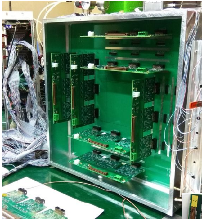
Back: Front End Electronics and triggering boards (custom)
