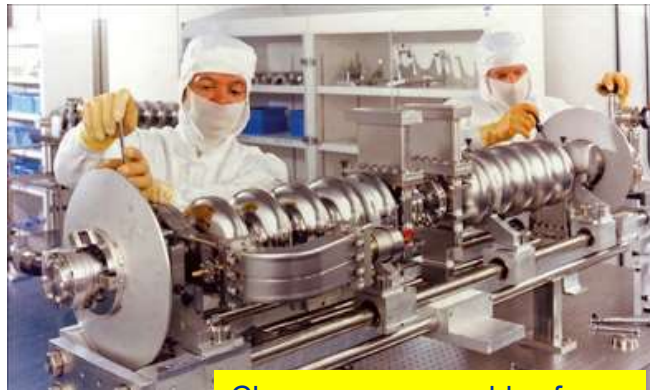
Clean room assembly of superconducting RF cavities
