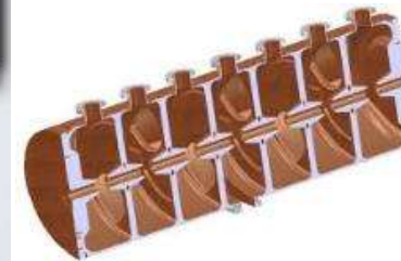
Multi-cell linac cavity (Linac4 120 MeV, 352 MHz)
