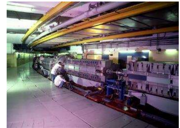
The CERN PS, 25 GeV, 200 m diameter
