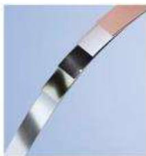
Fig. 1. A 12 mm tape produced by BHYS via IBAD and PBD method
