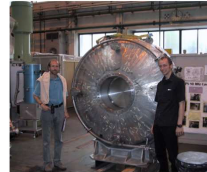
Single-gap cavity 88 MHz
