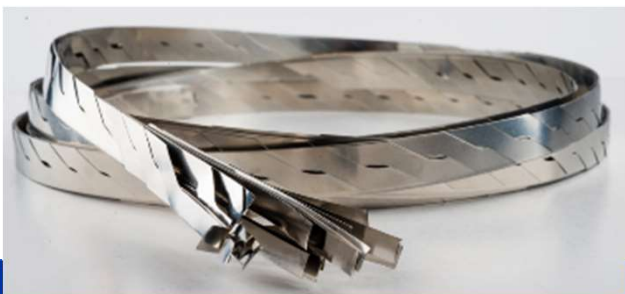
Fig. 1. A 12 mm tape produced by BHYS via IBAD and PBD method
