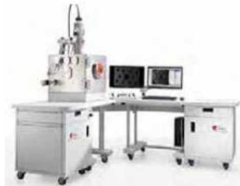
Fig. 4.8: A desk-top e-beam laboratory machine for welding and structuring with a magnified, backscattered electron-image.
