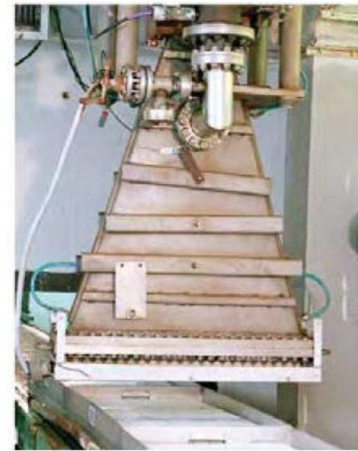
Fig. 4.12: E-beam technology for sterilising medical products
