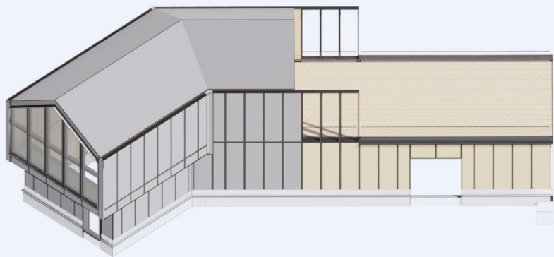
BIM model façade / roof modules - ENAR
