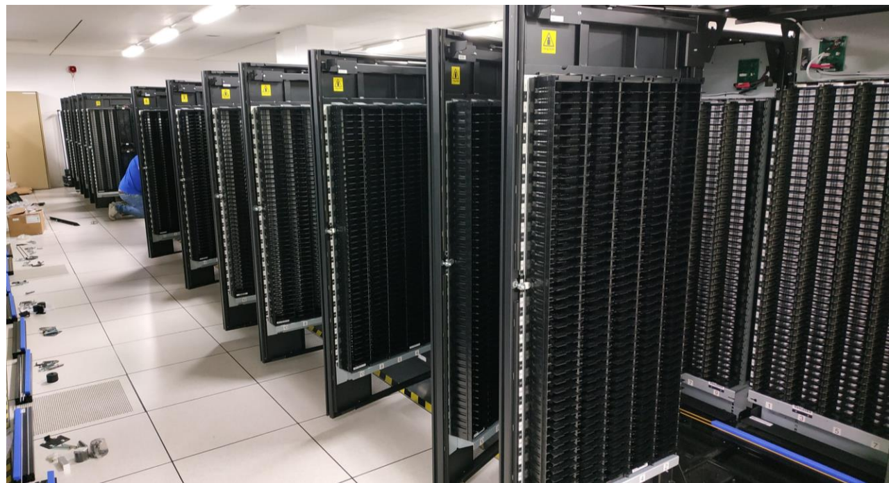
Tape storage for LHC data with capacity of 600PB provided by 6 tape libraries with 50 000 tape cartridges
