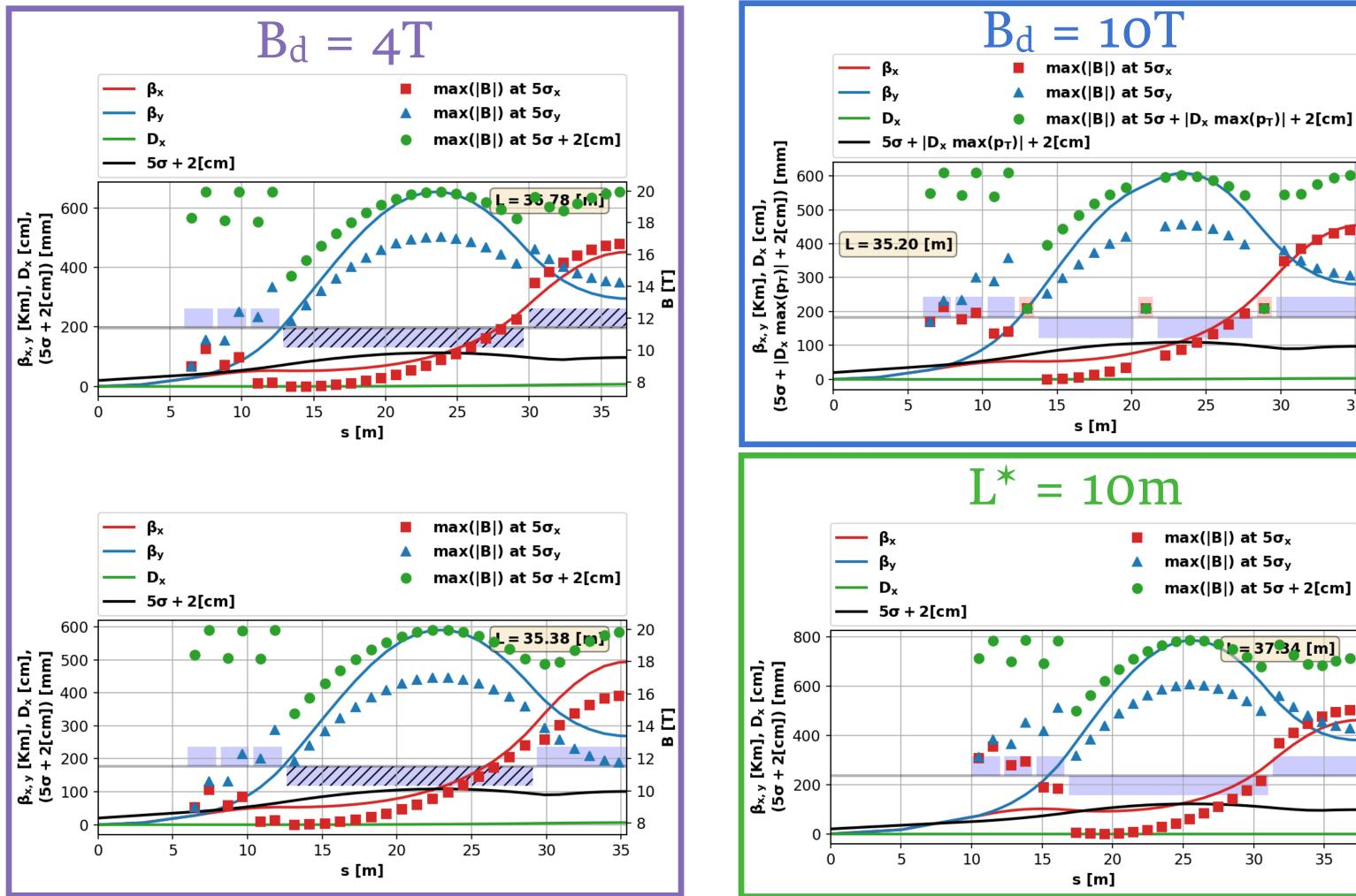
• For the vo.4 different FF schemes with dipolar components or an elongated L\* are designed for the mitigation of the Beam Induced Background (BIB) but without any significant contribution.
