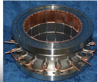
Tile-style SiC HOM damper (Courtesy: T. Schultheiss)
