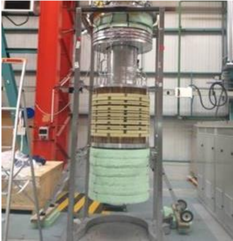
3 T field, 350 mm warm bore 350 ppm in a 300 mm sphere Operating cost: 15 k€ plus 6 k€/day
