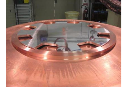
Stiff ring ready for e-beam welding
