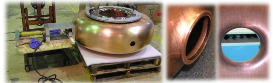
Cavity port extrusion 5
