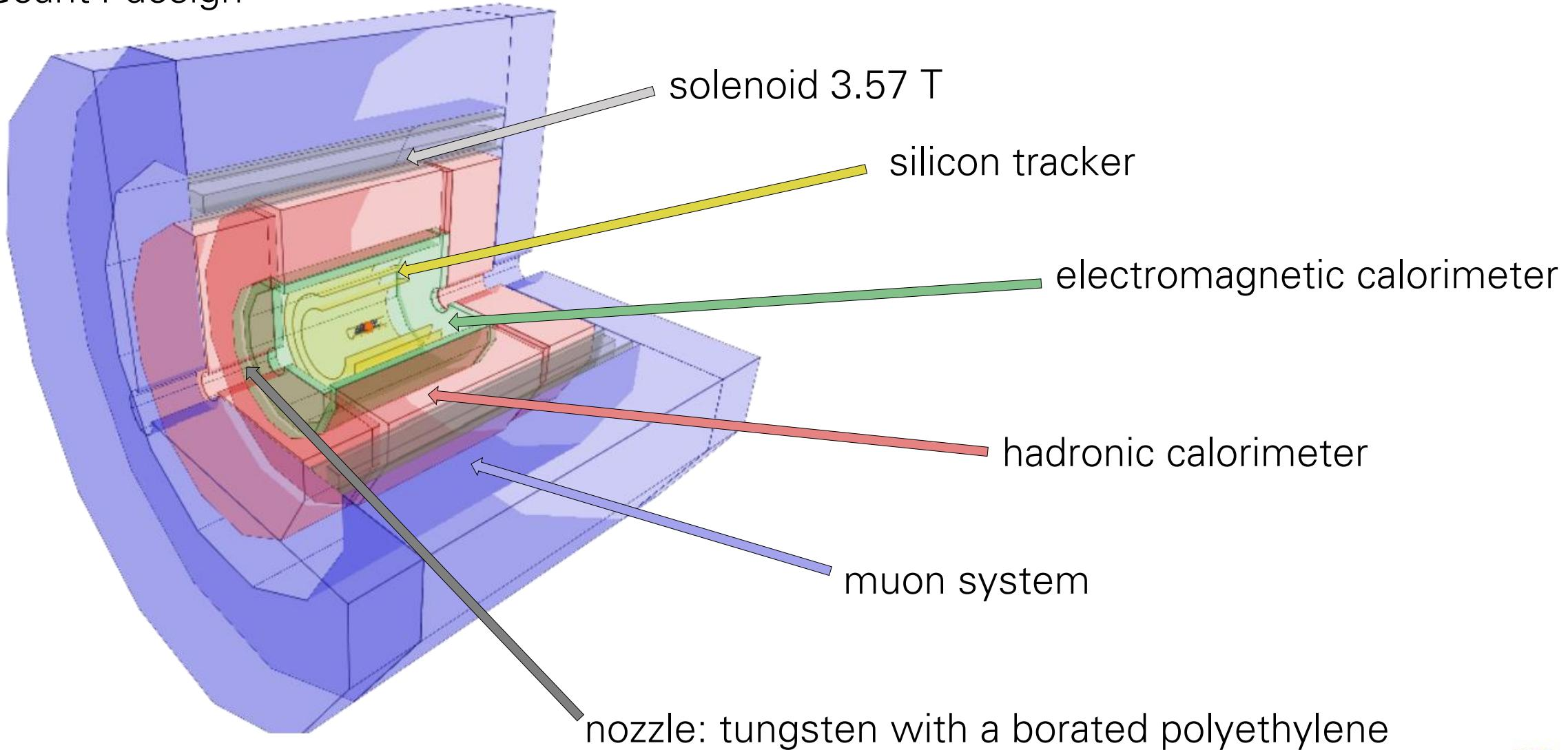
nozzle: tungsten with a borated polyethylene
