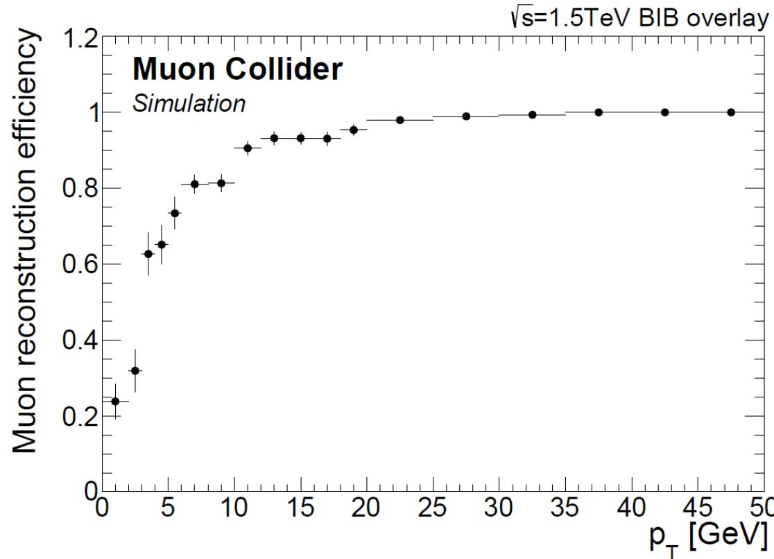
Efficiency and resolution as for single muon w/o BIB (CT track)
