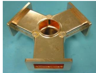
Figure 1: JLab Ampere class cavity with HOM loads and waveguide fundamental power coupler.
