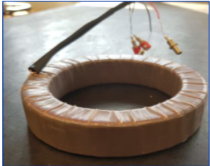
Vitroperm500F. Non-standard dimensions and very-high permeability (about 80,000)
