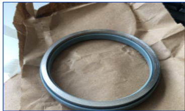
Mu-metal sample in the holder
