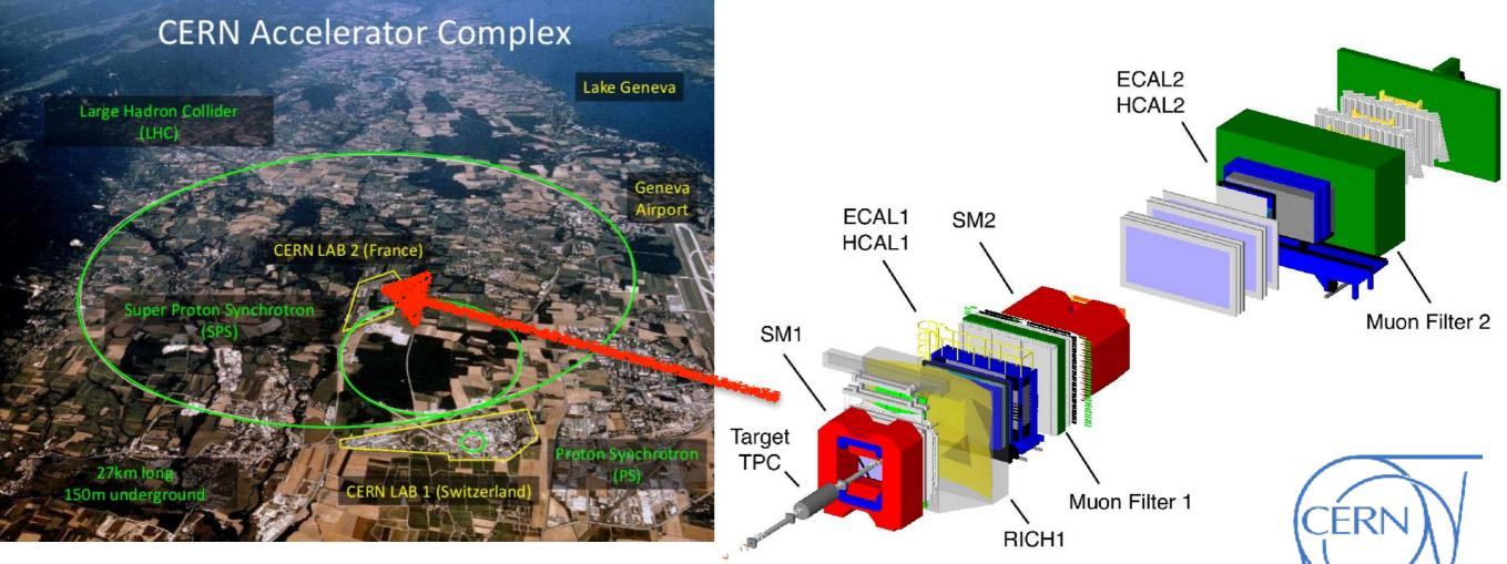
Use M2 beam in the CERN/SPS North Area Versatile beams (muons and hadrons of both charges) Beam momenta ranging from 50 - 280 GeV/c Intensity limited by radiation protection
