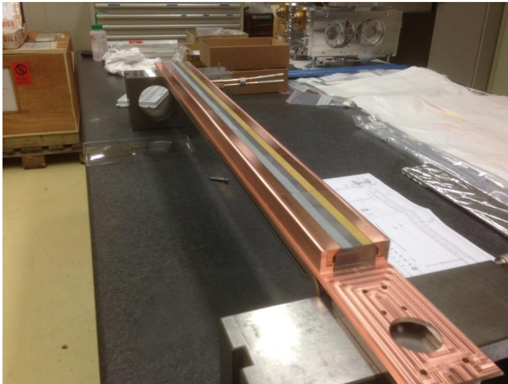
LHC collimator test jaw with 3 different surfaces to test with beam: Titanium nitride (yellow), Molybdenum (black), Molybdenum graphite (grey – bulk material).
