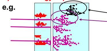
If these hits are clustered together with these, lose energy deposit from this neutral hadron (now part of track particle) and ruin energy measurement for this jet.
