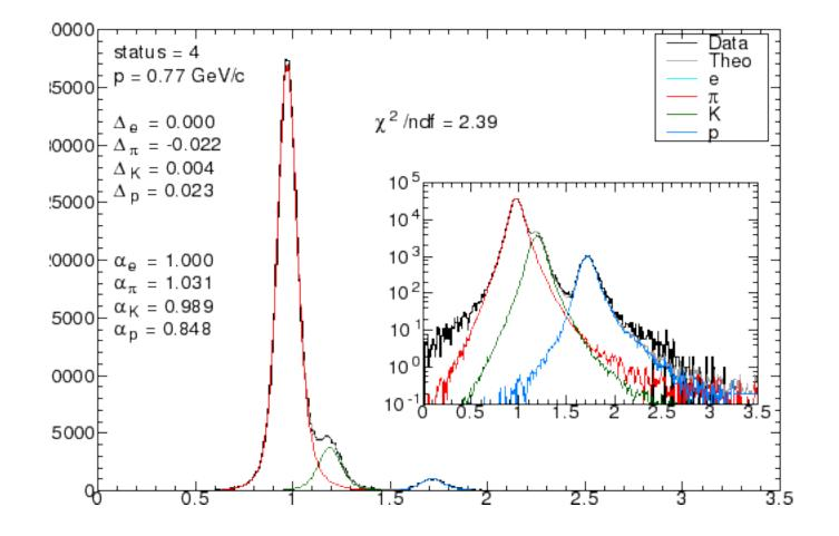
Sometimes only few hits on track  $\rightarrow$  Gaussian limit is too far Estimation of "average" dE/dx, with help of an analytical model
