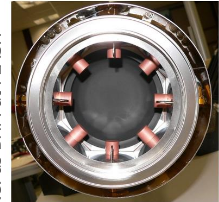
Figure 1: View of the BHM from the dump. The BHM sensors are inside the caps. Four loops of the magnetic-mean energy to create an coupled BPM are right in front of the BHM sensors.
