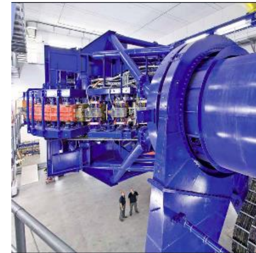
Heidelberg HIT C-ion gantry (600 tons)
