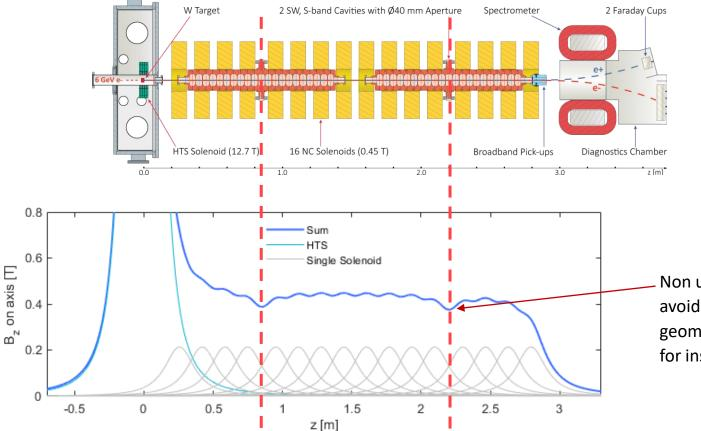
Non uniformities must be avoided. Constraint by physical geometry (e.g. waveguides, space for installation, etc.)
