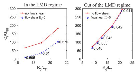
In the LMD: strong flow shear, significant suppression of turbulence especially near marginal stability
