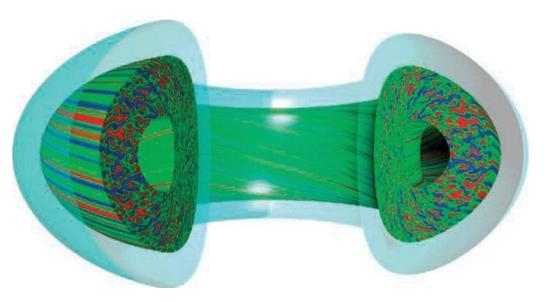
Microturbulence causes more than 90% of energy loss in tokamaks
