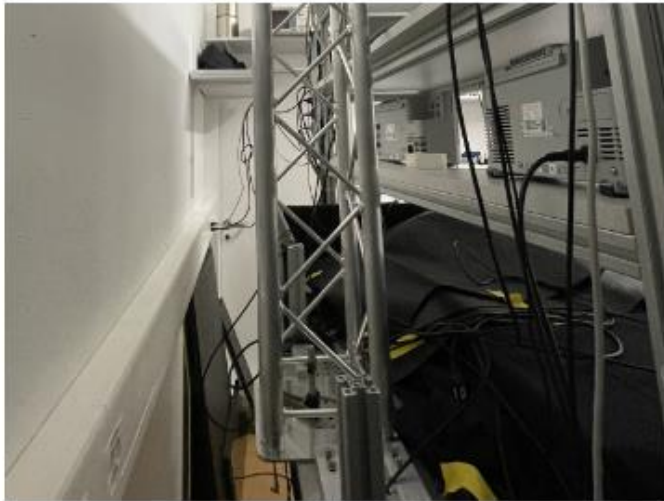
A tower sitting on the laser table supports an optical breadboard
