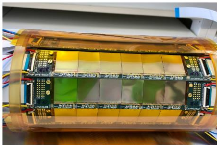
(e) Mounting of the helium confinement.
